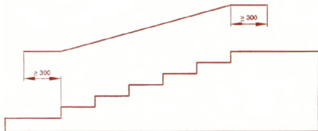
FIG. 16 EXTENSION OF HANDRAIL IN STAIRS
