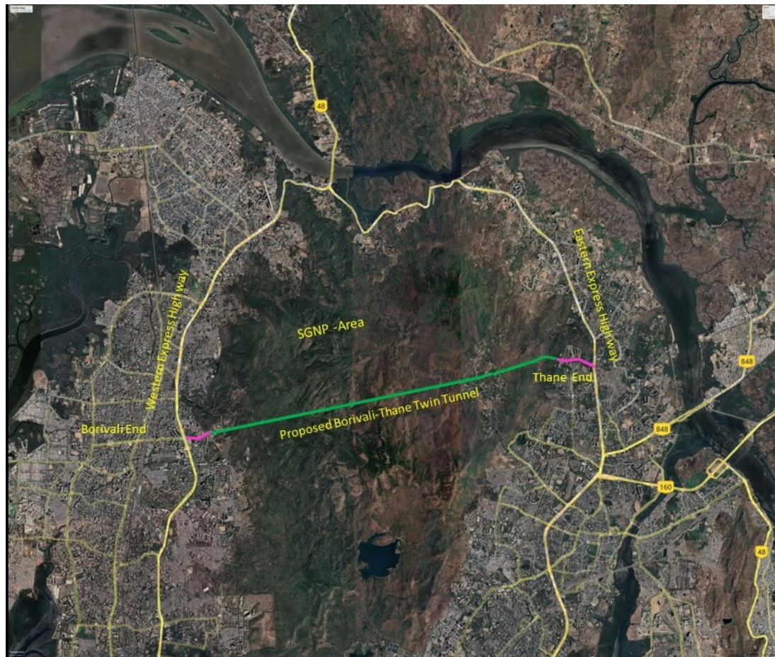
Figure2.1: - Study area showing existing road link and proposed connection between Thane - Borivali underneath Sanjay Gandhi national park
